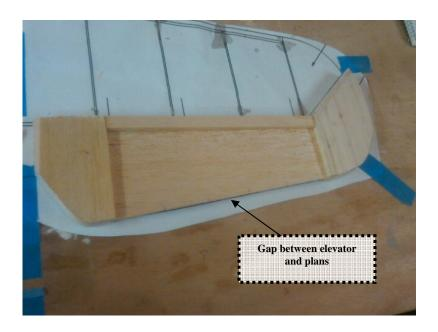
Find both root and tip elevator blocks (You might need to cut or sand to a rough shape).
