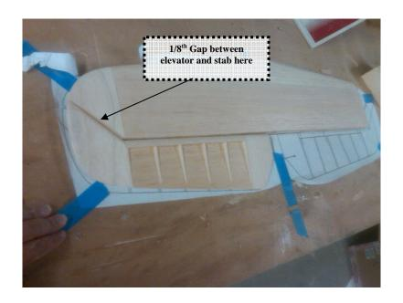
At this point you will glue the Stab Tip to the Stab. Sand to shape and check they fit. As you are sanding make sure the tip of the elevator and stab don't it and there is about a  $1/8^{\text{th}}$  inch gab between.
