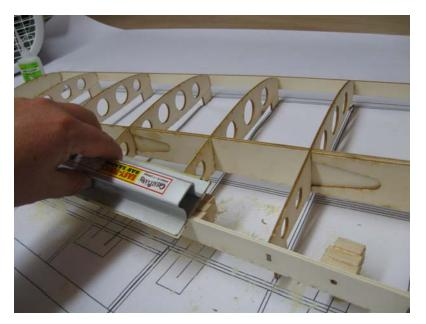
At this point, you will want to sand both TE, LE, and WS to fit the contour of your ribs.
