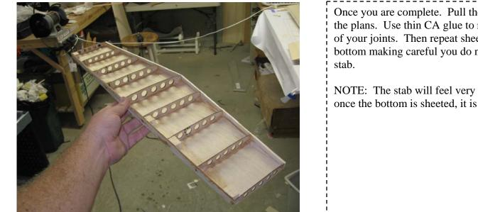
Once you are complete. Pull the stab off of the plans. Use thin CA glue to re-glue all of your joints. Then repeat sheeting on the bottom making careful you do not warp the
