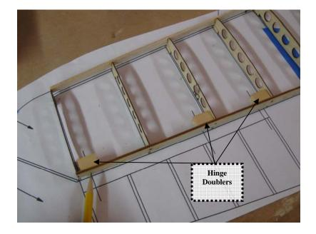
Use Scrap Wood to glue as "doublers" for your hinges. Lines are dawn on the plans that show hinge lines. Do this to both sides of your stab.
