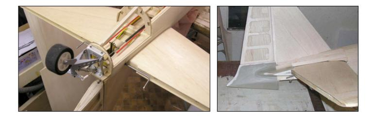
• Another example below. This uses an air cylinder to retract the tail wheel. Note that at this stage all the balsa was removed and F10 cut out to gain access. The tail wheel assembly is mounted using 2 pieces of hardwood. The pic also shows the lip where the tail cone goes so that it finishes flush with the fuselage.
