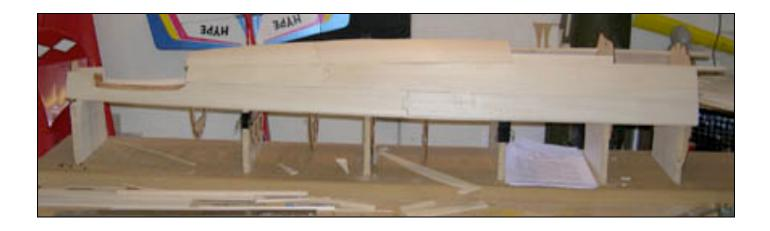
• Once you have sheeted the top of the fuselage you can remove it from the jig. You then need to install B1A to the backside of the firewall. This piece is to help form and glue the wing saddle doublers, FS4A (sheet 3).
