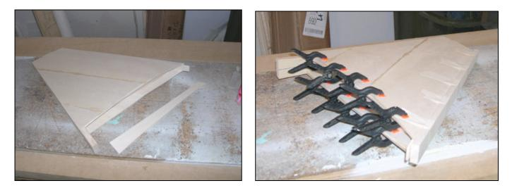
All surfaces on the full size had a trailing edge thickness of 1/16<sup>th</sup> meaning that careful sanding is required to duplicate this.
