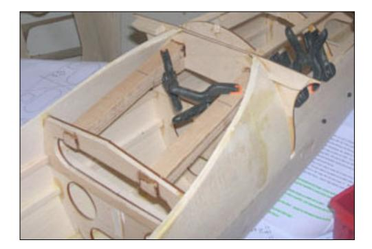
• You can the put the wings back on and drill through the wing and blocks to locate the wing making sure it is square to the fuselage.
