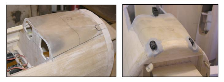
• The cut outs in the dash board are for the machine guns. These again would be easier to do before the model is constructed but careful use of a dremmel does the job.
