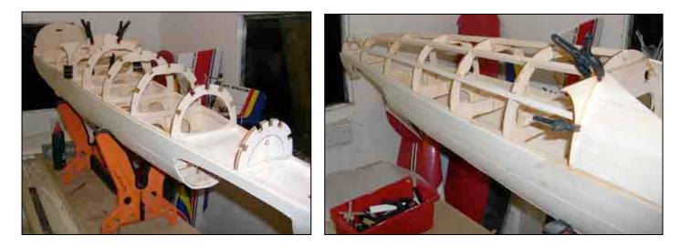
• Remember that before you sheet the whole fuselage you need to think about how the back end is going to be controlled i.e push rods, air lines, closed loop wires etc. It is beneficial to leave access through the bottom of the fuselage until the last minute.
