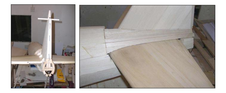
• After sanding the fillets to shape they need raising to simulate the full size. This is done either with filler or outlining with ply and the inner filled with balsa.
