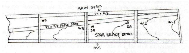
6. Make sure you keep all the ribs at 90 degrees EXCEPT W-1. Install the false spar by cutting pieces of the ½ x 5/8" stock and placing the pieces in the space between the ribs. These pieces are placed on top of the "spar brace". Install the top spar. Make sure all the ribs remain flat on the table. If the trailing edge of a rib appears lifted, make your adjustment now Install the 1/8" shear webbing to front & rear of the spar W-1 & W-12.
