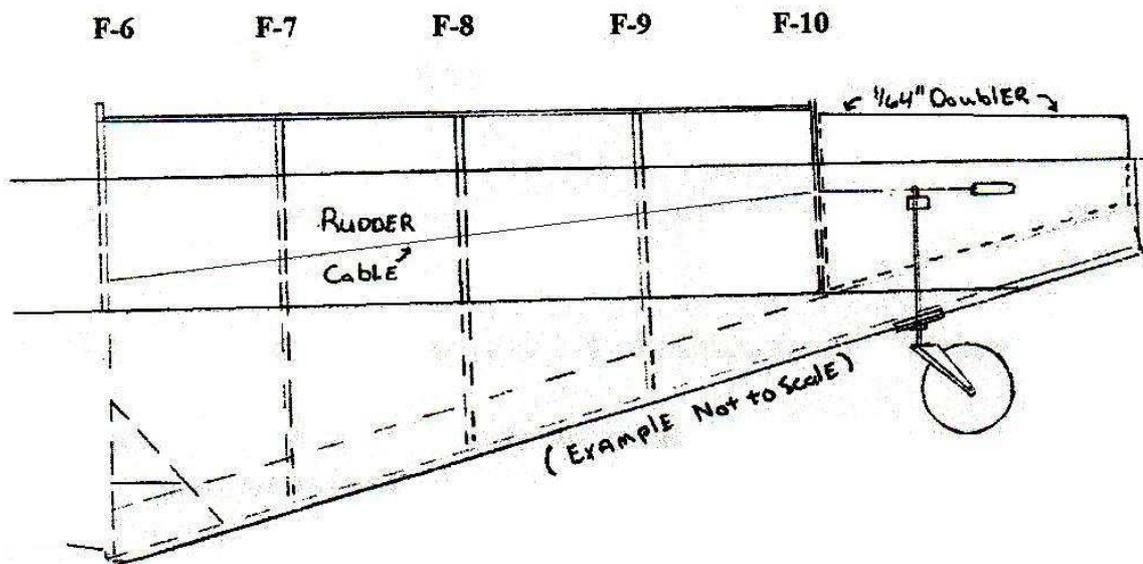
14. The stringer at the top of FS-1B should end at F-10. Now before you add F-S4A make a  $\frac{1}{64}$  or  $\frac{1}{32}$  ply doubler, which goes from F-10 to the rear of FS-1B. The doubler should stick up above FS-B so it will be flush with the top of FS-1B when it is put in place. There should be a doubler placed on both sides.
