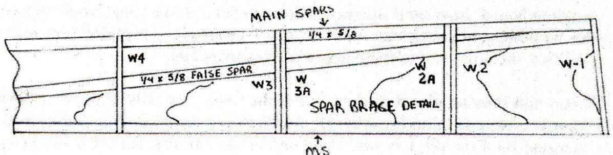
6. Make sure you keep all the ribs at 90 degrees EXCEPT W-1. Install the false spar by cutting pieces of the 1/4 x 5/8" stock and placing the pieces in the space between the ribs. These pieces are placed on top of the "spar brace". Install the top spar. Make sure all the ribs remain flat on the table. If the trailing edge of a rib appears lifted, make your adjustment now. Install the 1/8" shear webbing to front & rear of the spar W-1 & W-12.
