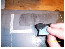
I then wipe this mixture on the entire aircraft. Front to back on the wings and stab, and top to bottom on the fuse and vertical fin. I don't do the entire plane at once, I will work in sections at a time. When wiping the black mixture on the plane, I will make sure I get it into all the rivet detail, hatches, panel lines etc that I want to highlight. After about a minute or less, you can then wipe the mixture off.
