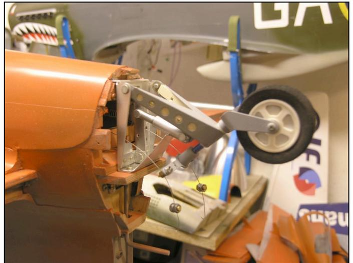
The tail wheel on the right above is a lightweight plastic wheel with a foam tyre which was put in a drill chuck and sanded down to a scale flat section.
