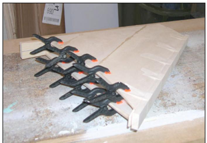
**All surfaces on the full size had a trailing edge thickness of  $1/16^{\text{th}}$  meaning that careful sanding is required to duplicate this.**
