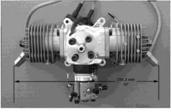
Slant-Plug Configuration: Plug-Cap to Plug-Cap = 10"
